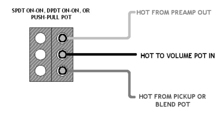
NOTE: Most ACTIVE pre-amps use low impedance pots, (10k-100k). It is recommended to use 100k-250k pots with this mod.
