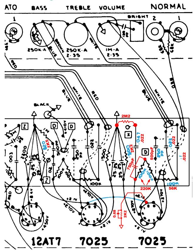
Blue VALUES replaced by values in RED Blue COMPONENTS removed from circuit Red components added to circuit
