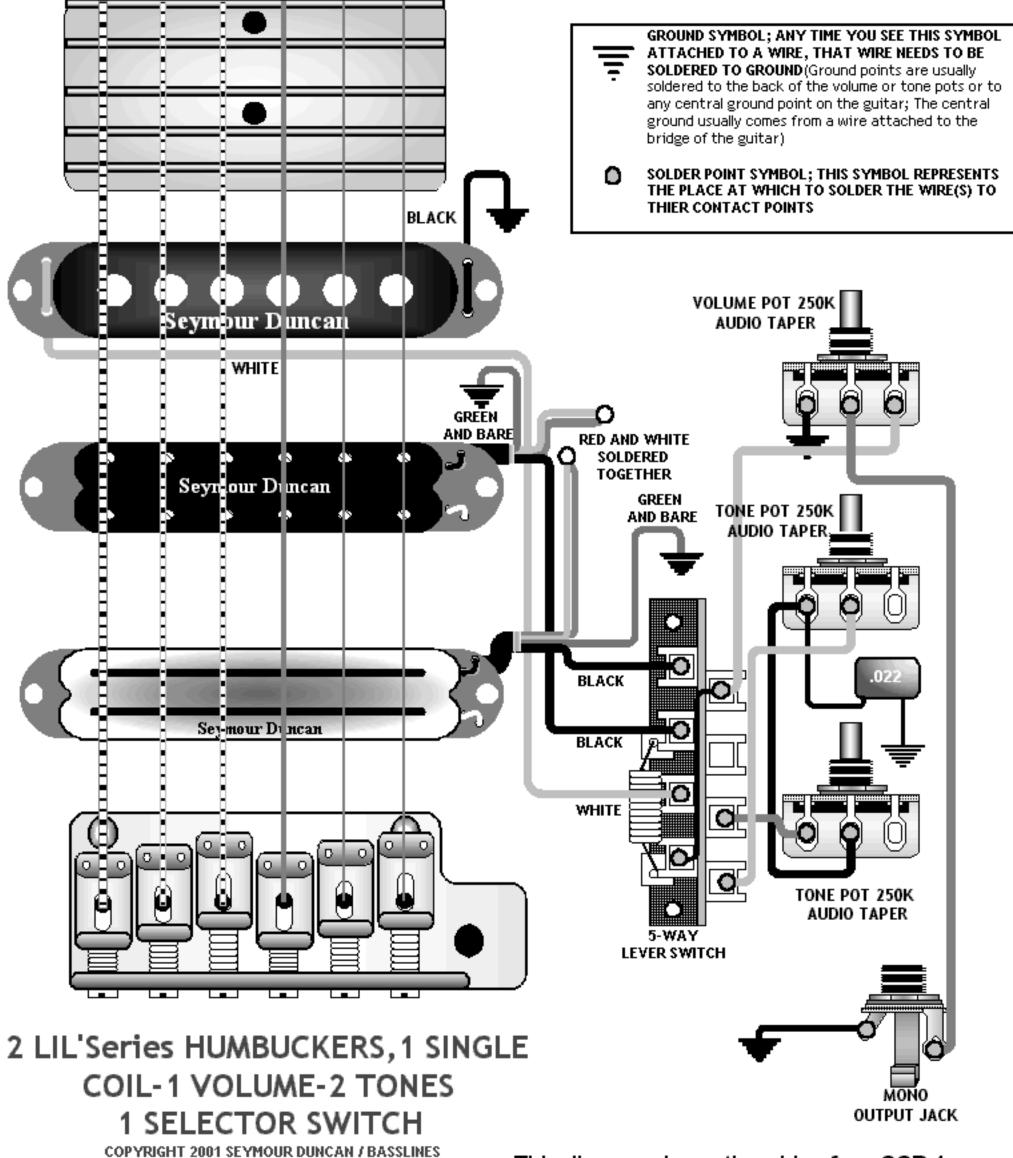
This diagram shows the wiring for a SCR-1
